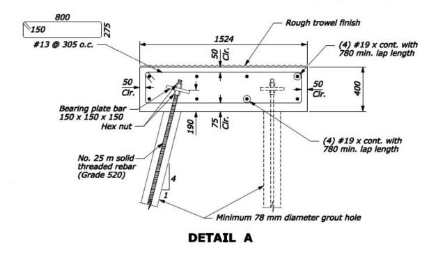
Figure 5 – Micropile Cap Typical Detail
